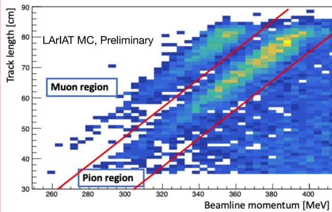
Initial precuts on beam momentum, Bragg peak, start and end positions of the primary particle.
