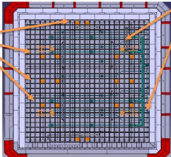
8 PMTs looking towards the field cage at the same distance than the X-ARAPUCAs and at the same height for the PDE measurement (6 TPB + 2 PEN PMTs).
