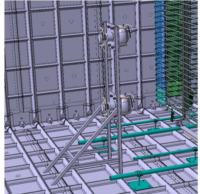
PMT layout in ProtoDUNE-VD
