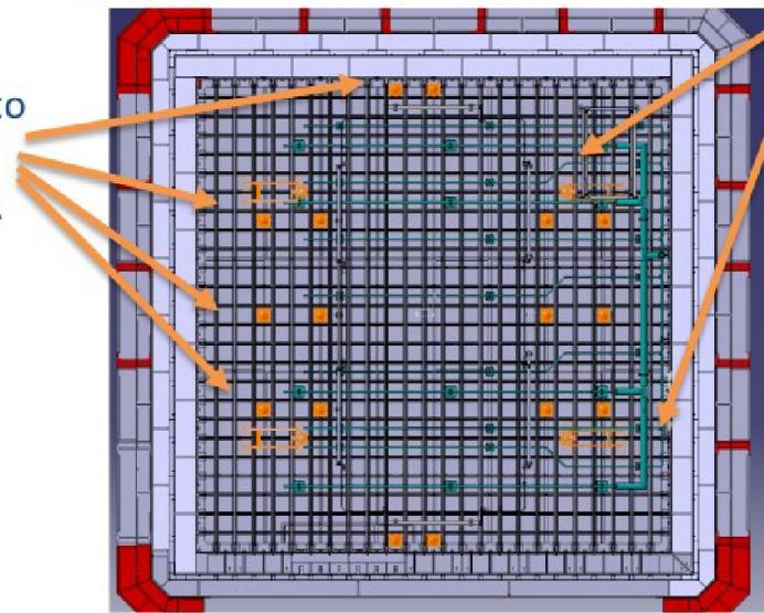
8 PMTs looking towards the field cage at the same distance than the X-ARAPUCAs and at the same height for the PDE measurement (6 TPB + 2 PEN PMTs).
