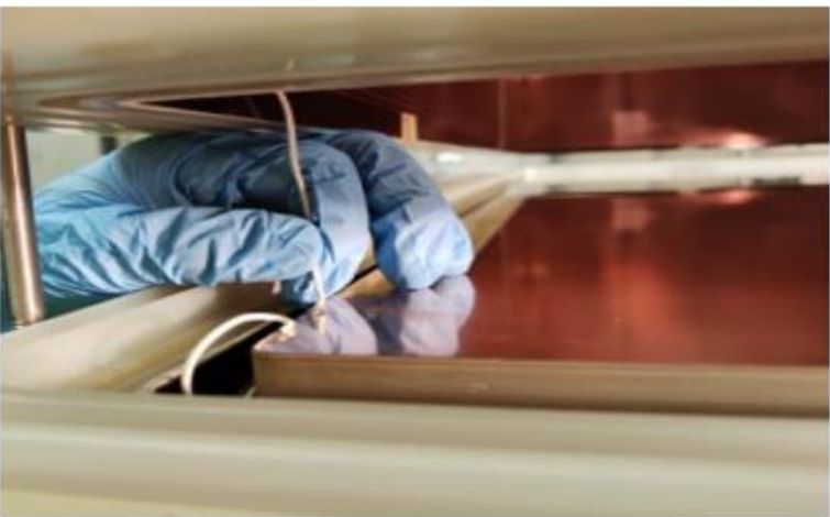
Connection of last strips to cathode and to high voltage feedthrough
