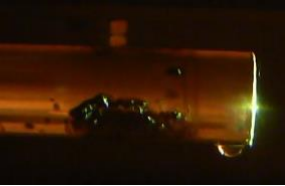
MINOS NT-01 target containment water leak (FNAL)
