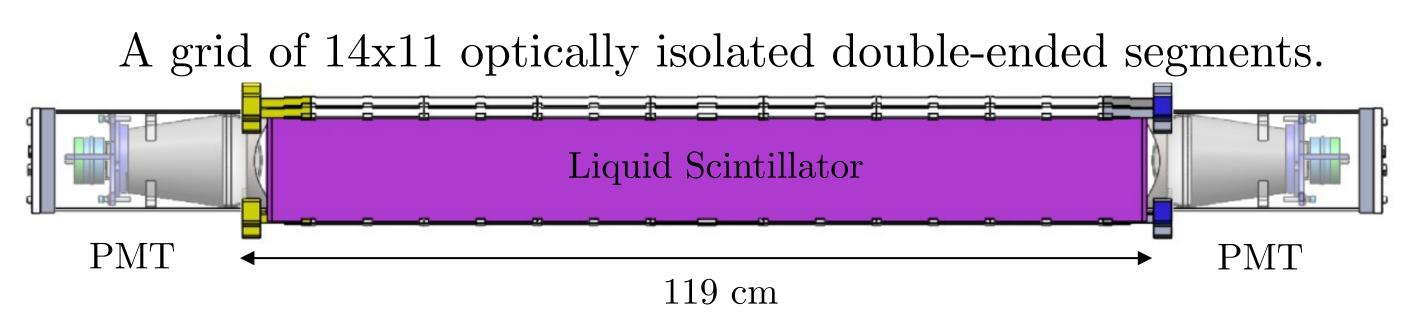
The ingress of liquid scintillator into PMTs led to the failure of some PMTs, resulting previous results to be dominated by statistical uncertainty.
