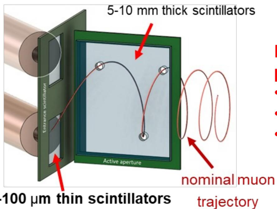
Provides trigger signal of storage pulse kick
