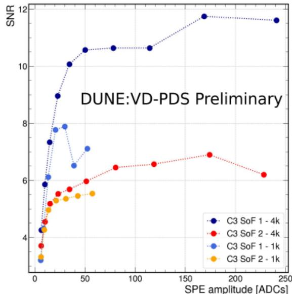
Varying the gain withing DAPHNE modifies the amplitude of the SPE, and affects the SNR.
