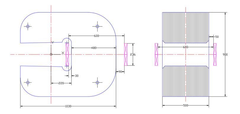
Laminations from M15 low carbon steel have 0.5 mm thickness. At magnet core ends placed stainless steel plates of 10 mm thick (not shown). Longitudinal rods should be electrically insulated from laminations. Dimensions in mm to start the mechanical design.
