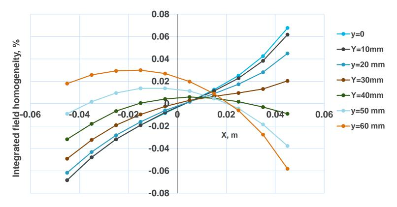
Integrated field V29: 0.16692 T-m Integrated field homogeneity +/- 0.07 % (spec. +/- 0.1 %) in the good field area x=+/- 45 mm, y=+/- 60 mm.
