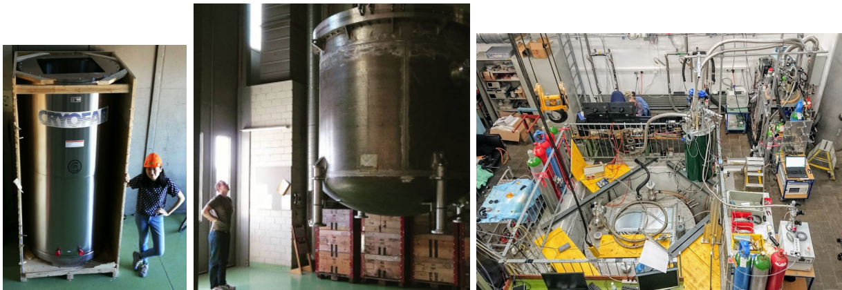
Figure 1.77: (Left) The cryostat for testing individual LArTPC modules for the 2x2 Demonstrator (Center) The cryostat for the ArgonCube 2x2 Demonstrator (Right) The 2x2 cryostat and cryogenics system at the Univ. of Bern.
