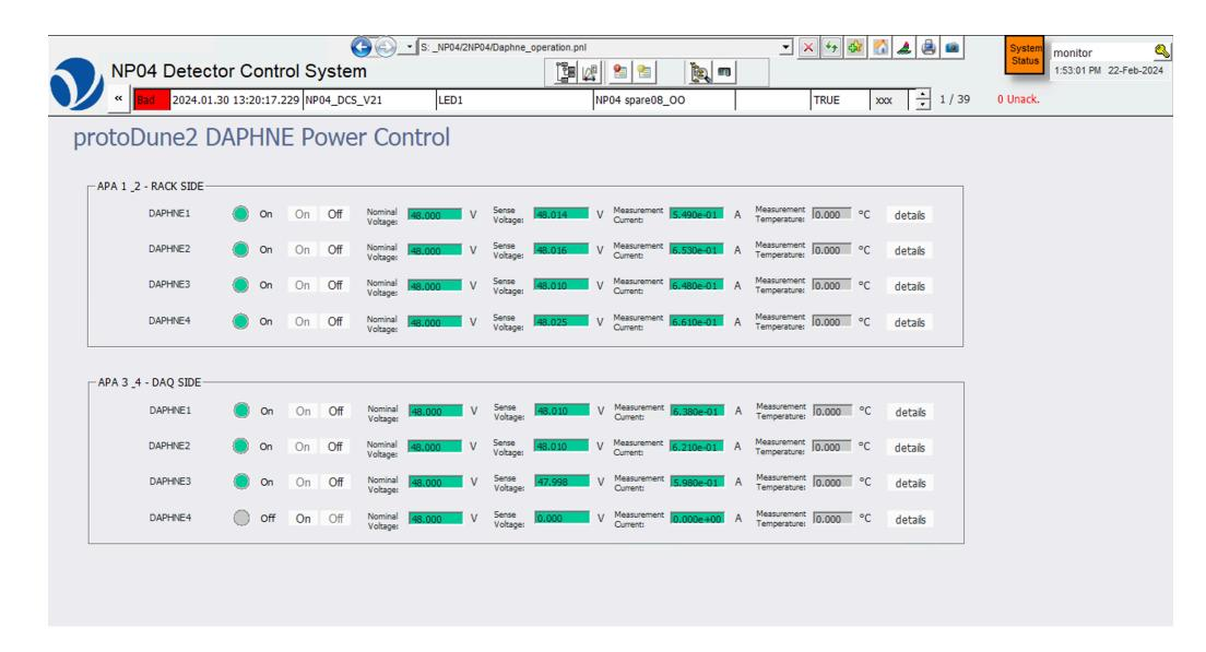
No hardware interlock for purity monitors (PrMs) possible at this moment, instead a button indicating powered SiPMs will be added to the DAPHNE power control panel. Current PDS expert should manually take care of this button, which will prevent PrM operation. Ongoing discussions with Jianming and Xavier
