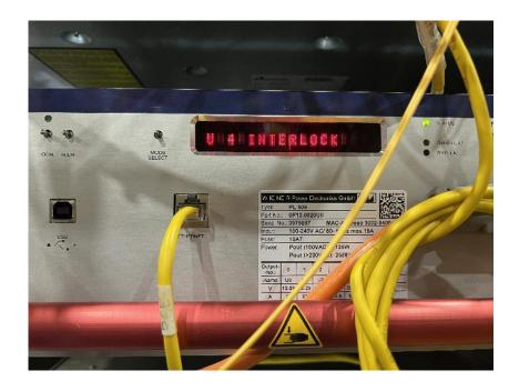
If 1/4 Fan is OFF and Temperature of WEIC crate goes above certain trip limit the DUNE-CE-Interlock will turn the 48 V power to the PTC OFF (All WIBs, FEMBs will go OFF)
