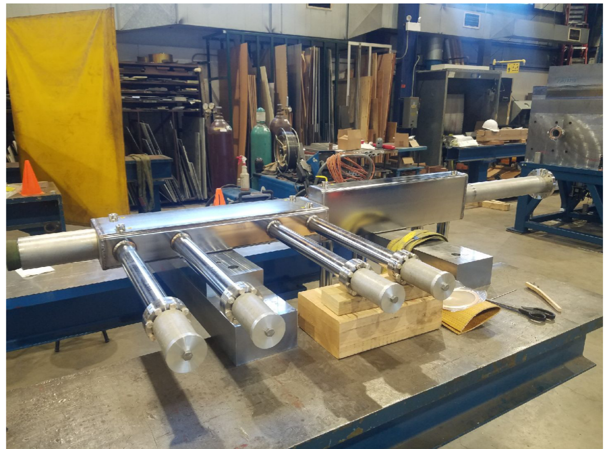
Booster secondary collimator vacuum chamber
