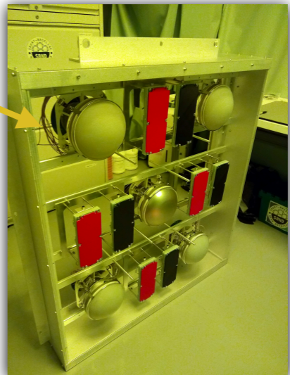
Photo Detection System: 120 PMTs, 192 X-Arapucas
