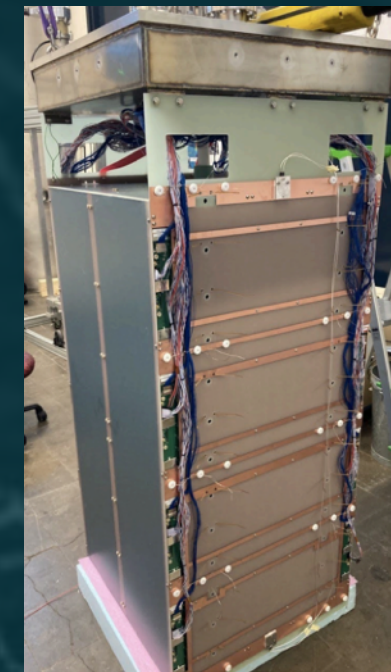
LArPix Tile with VUV SiPM read out by LightPix
