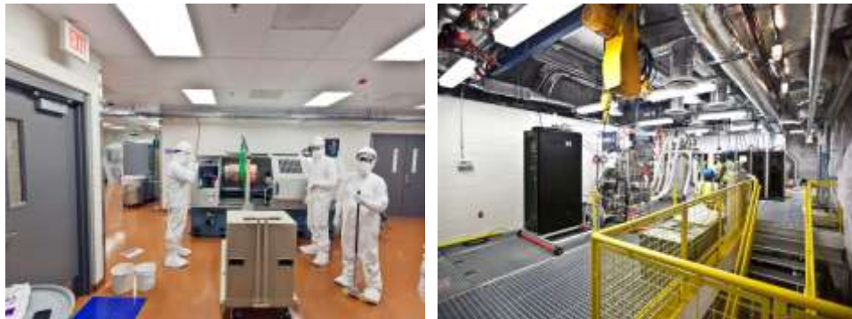
Figure 4. Sanford Underground Research Facility: Billet of radiopure electroformed copper for the Majorana Demonstrator experiment on a lathe in a clean room at 4850 ft depth (left); LUX experiment at 4850 ft (right).
