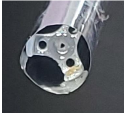
3D Printed spacers inserted in straw tube
