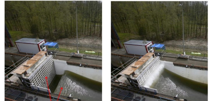
Membrane Wall with Wave Approaching
