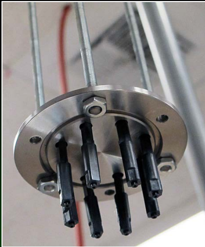
SiPM housings/ferrules mounted on cold frame
