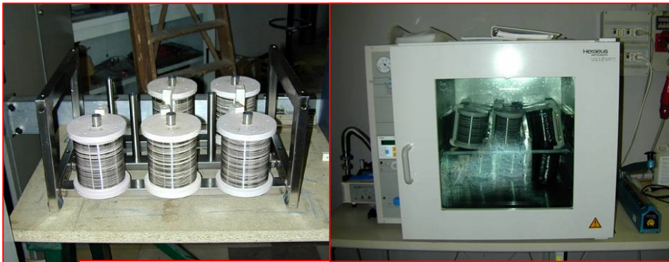
PVC spools after washing and during drying
