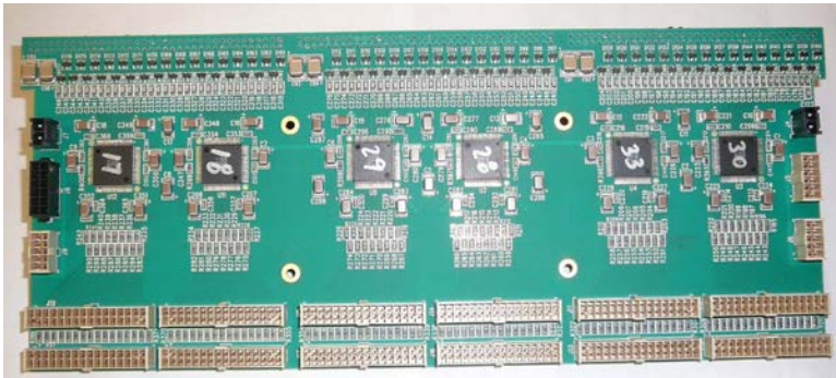
Horizontal cold mother board with 12 ASIC chips (192 channels) populated
