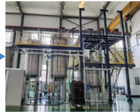
Mixing LAB with PPO and bis-MSB
