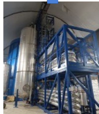
4) Gas stripping to remove Rn and O 2
