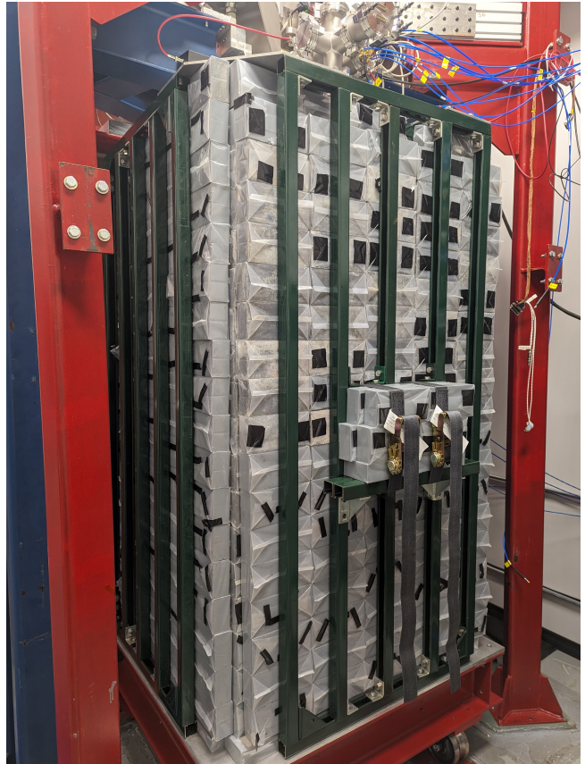
Figure 5. A photo of the lead shield encapsulating the dilution refrigerator used in NEXUS. The scintillators will lay inside the shield below the refrigerator.
