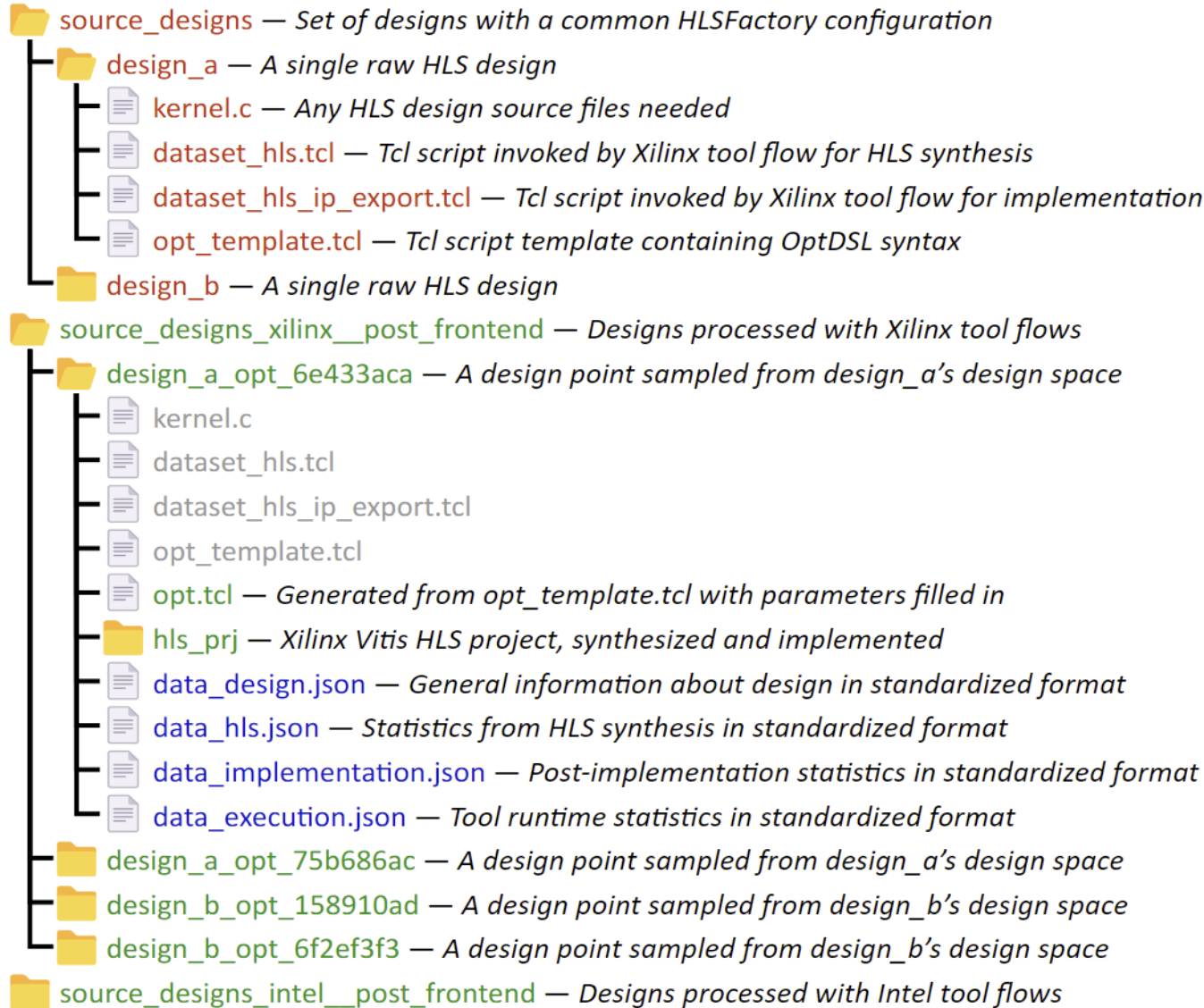
Fig. 4. The directory structure that HLSFactory uses. Red are input files; green are the intermediate design points; blue are output files.
