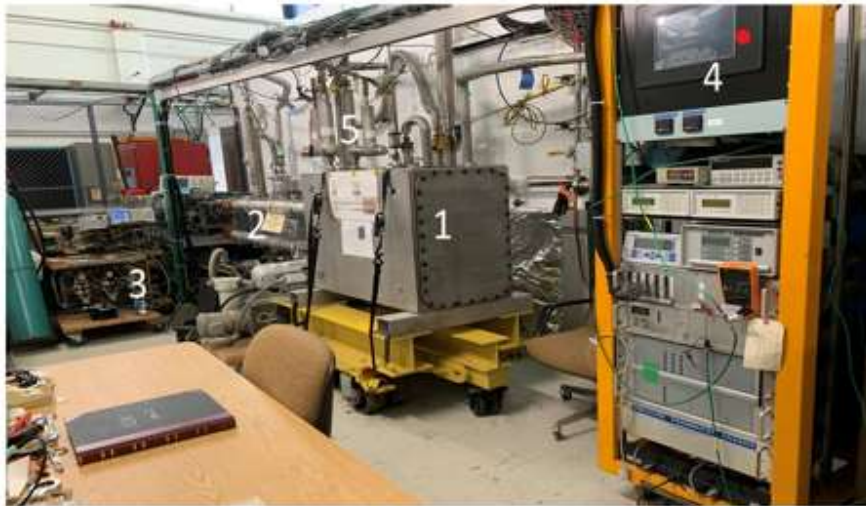
1 - Magnet, 2- Current leads, 3- Power supply, 4 - Control electronics, 5- Liquid Helium lines
