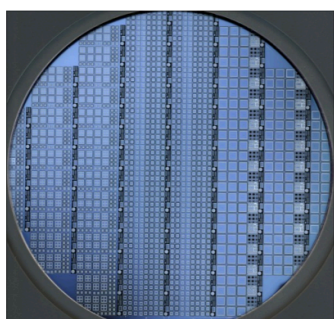
prototype with new LGAD design funded by INFN-CSN5 and AIDAInnova grants
