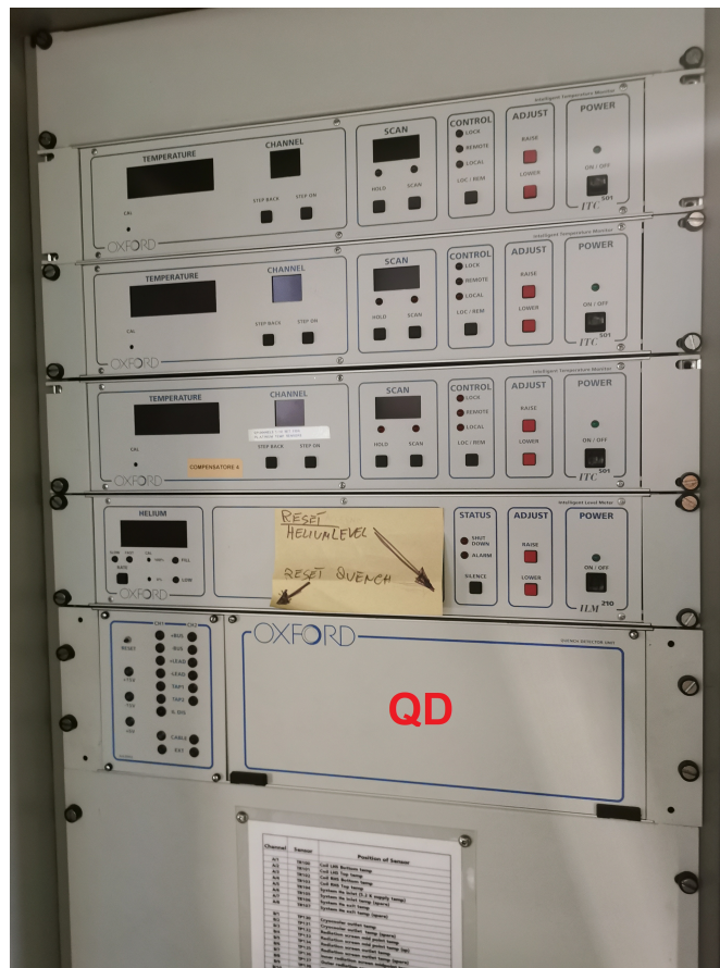
Figure 1.66: Kloe Magnet Diagnostic Rack. The Quench Detector (QD) is marked in red.
