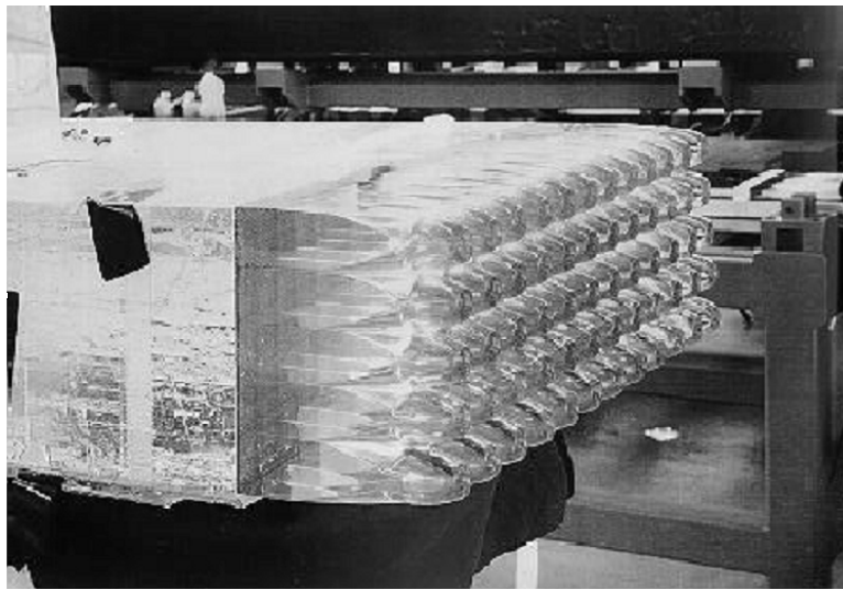
Figure 1.3: Light guides at one end of a KLOE ECAL barrel module before PMT installation.
