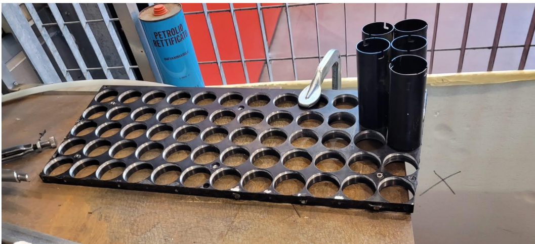
Figure 1.60: The aluminum grid supporting PMTs going to be replaced.
