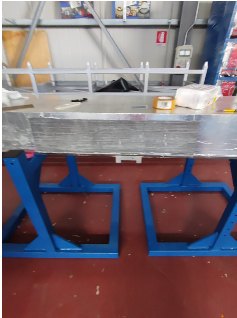
Figure 1.61: A module during the tape wrapping work.
