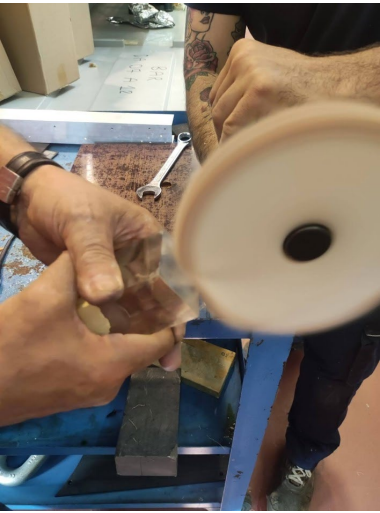
2 light-guides unstuck in 1 module have been polished and glued
