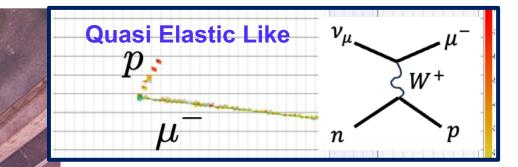
[LEFT]: One of three views We see several hits per particle to make tracks We use final state particles to reconstruct neutrino energy
