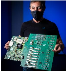
Fermilab's open-source Quantum Instrumentation Control Kit (QICK)
