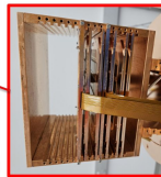
50 g (120 g) skipper-CCD array with 7 (16) layers (21.6 MPix each)
