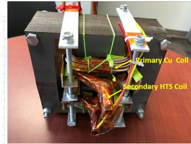
HTS Dipole (2022). 4 kA current in HTS coils circulated 12 hours without decay and a power source
