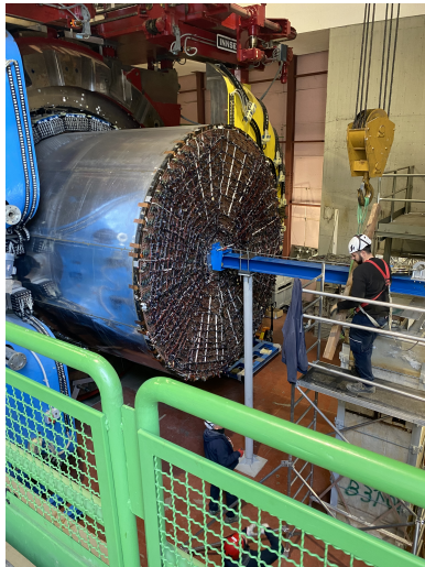
Figure 1.5: Left: extraction of the drift chamber at LNF. Right: zoom on the HEA200 beam and the trolley (detail in the text).
