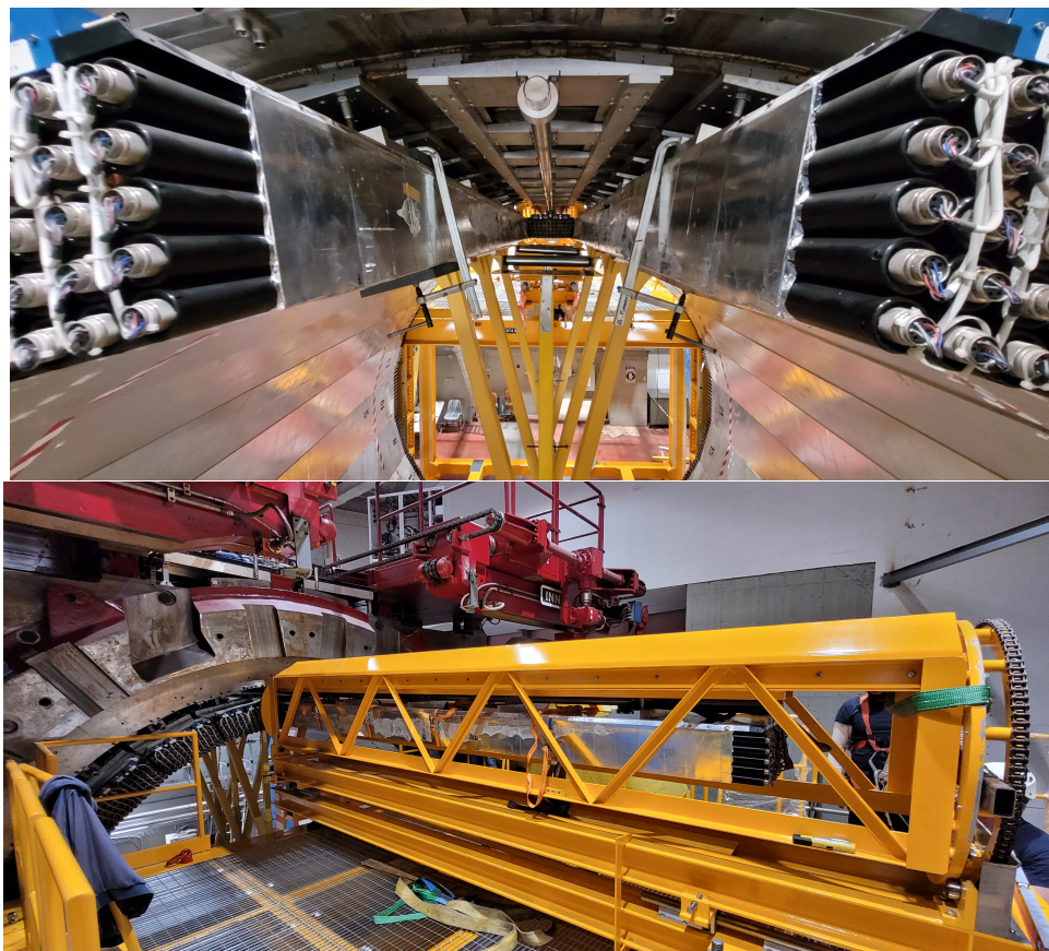
Figure 1.8: Extraction of the first barrel module from magnet cryostat.
