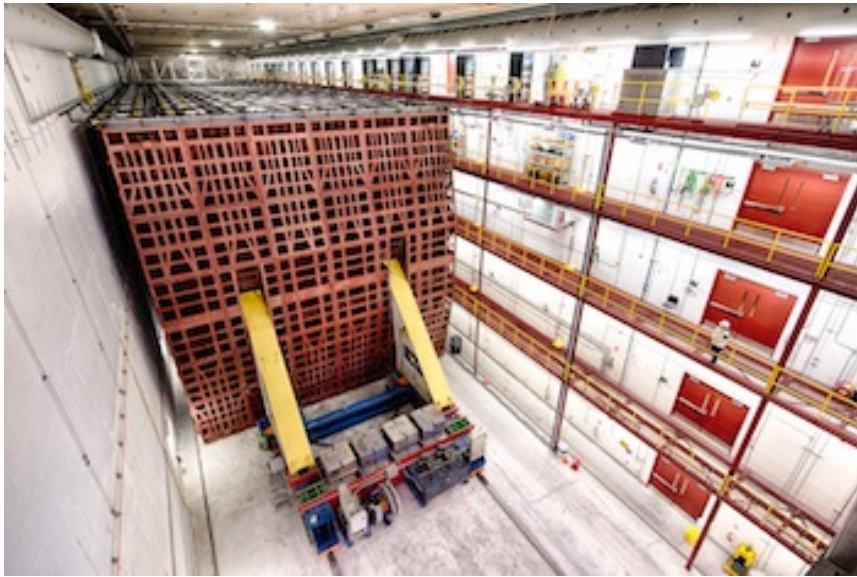
NoVA 14-kiloton far detector comprised of liquid scintillator
