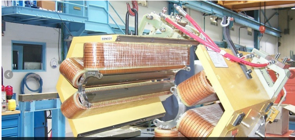
At the Magnet Systems Department we designed and fabricated many quadrupole magnets. Shown here is a Skewed Sextupole Magnet (SSM) during assembly.
