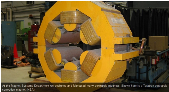
At the Magnet Systems Department we designed and fabricated many quadrupole magnets. Shown here is a Skewed Sextupole Magnet (SSM) during assembly.
