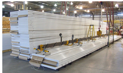
Highly reflective plastic extruded tubing 15.5-m long. Inside the detector, the tubing will be filled 2.7-million gallons scintillating oil
