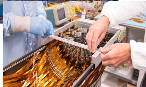
Quarter-section of the CMS Forward Pixel (FPiX) Detector Upgrade, part of LHC at CERN
