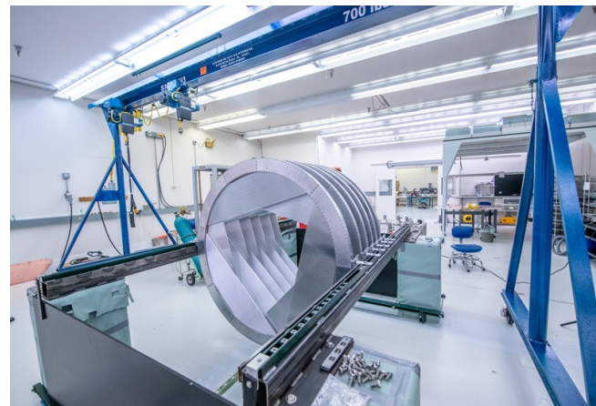
Stations of the Straw Tracker. The completed tracker will have 20 stations that will hold a total of 23,040 straws.
