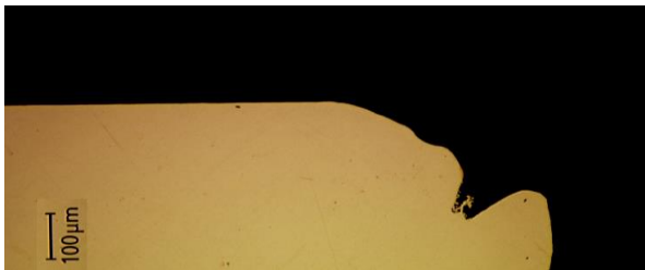
Damaged CLIC structure iris
