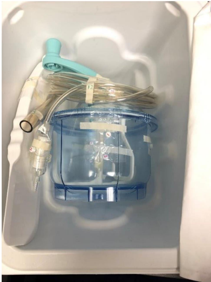
Figure 6: Top view; Photo of dosimeters placed in original dose-map sample
