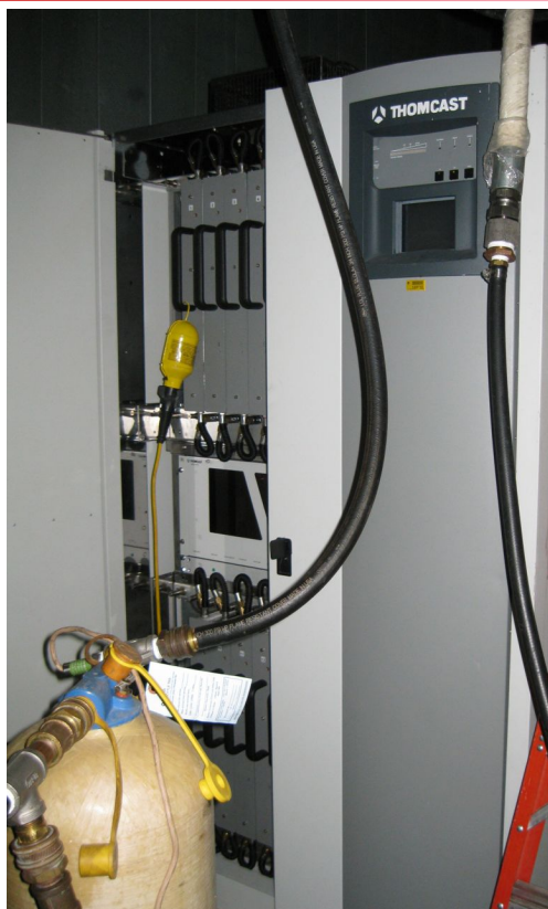
Thomson 10 kW Solid-state amp for testing HWR couplers at Argonne
