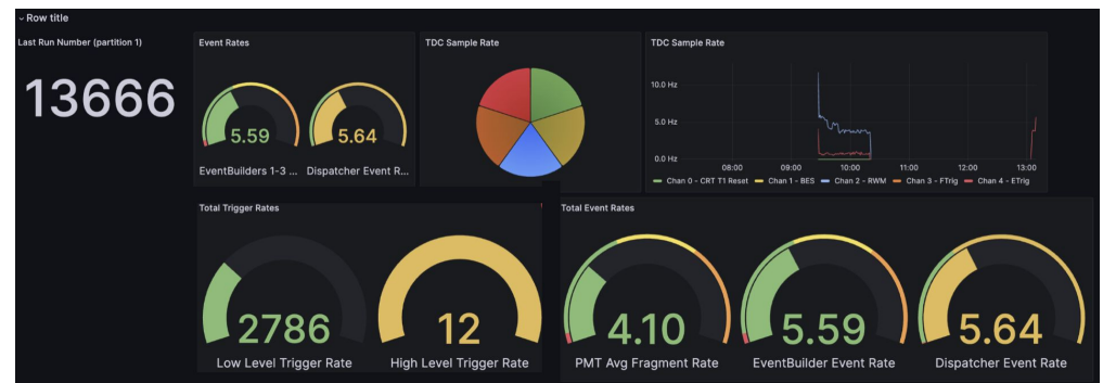
Monitoring of a recent run incorporating the light-based trigger logic, showing the trigger and event-building rates in real time
