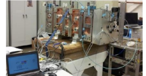
Bead pull measurement
