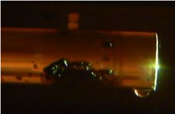
MINOS NT-01 target containment water leak (FNAL)
