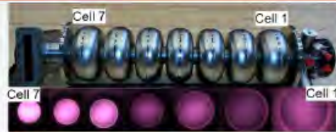
CEBAF C100 cavity with argon-oxygen plasma in each of the 7 cells
