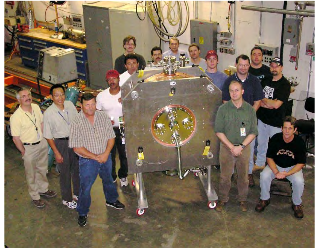
First 200 MHz cavity welded and EP'd by Jlab. Assembled in clean room
