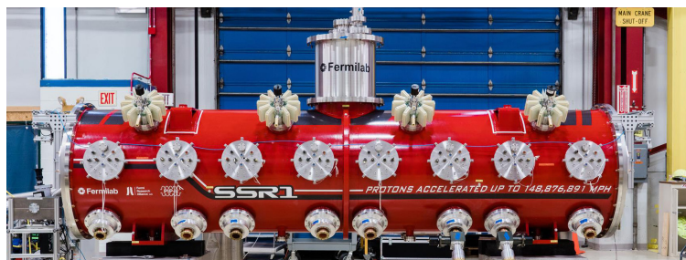
This photo shows the first PIP-II superconducting cryomodule, SSR1, built and successfully tested with beam at Fermilab, an example of the technology that will enable the Fermilab accelerator complex to generate powerful particle beams.
