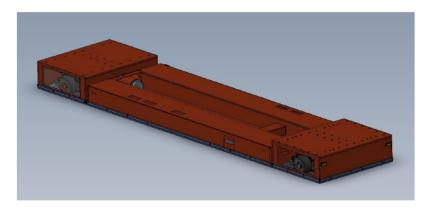
The manually guided vehicle (MGV's) captured in this proposal is equipped with modular traction/steering drives that are bolted to a fabricated steel frame.
