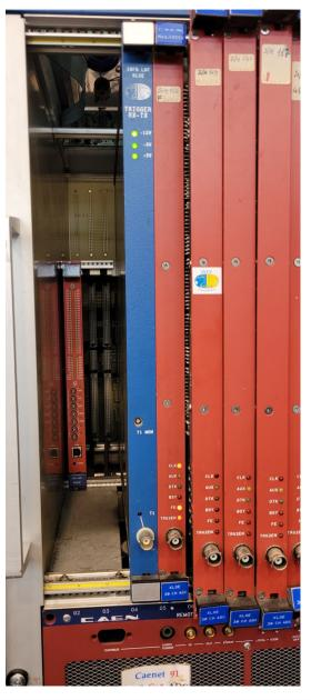
Power on of VME 9U crate with KLOE ADC and TDC boards (30 ch/board) + trigger distributor
