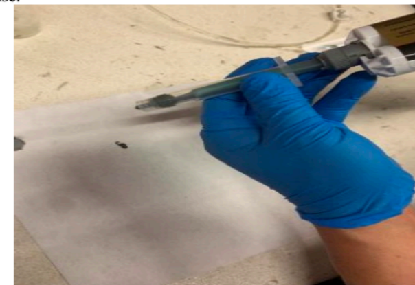
Figure 6: Filling a barrel with Epoxy
