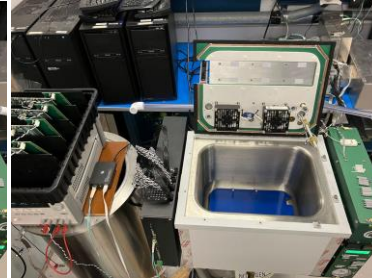
Remove FEMBs (Cold cables) one by one and put them into an ESD-safe Tray
