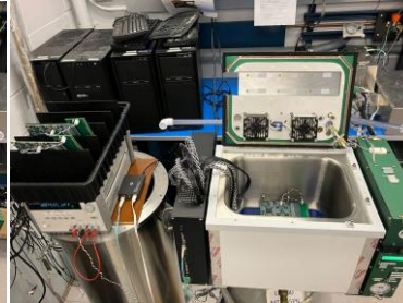
Remove FEMBs (Cold cables) one by one and put them into an ESD-safe Tray
