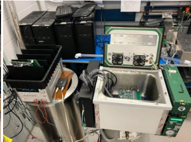
Remove FEMBs (Cold cables) one by one and put them into an ESD-safe Tray
