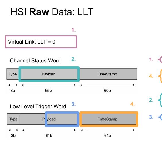
word t version : 6, detector id : 6, crate : 10, slot : 4, link : 0; word t timestamp low : 32; word\_t timestamp high : 32; word\_t raw\_input\_low : 32; word\_t raw\_input high : 32; word\_t trigger : 32; word t sequence : 32;
