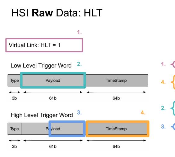
word t version : 6, detector id : 6, crate : 10, slot : 4, link : 1; word t timestamp low : 32; word\_t timestamp high : 32; word\_t raw\_input\_low : 32; word\_t raw\_input high : 32; word t trigger : 32; word t sequence : 32;
