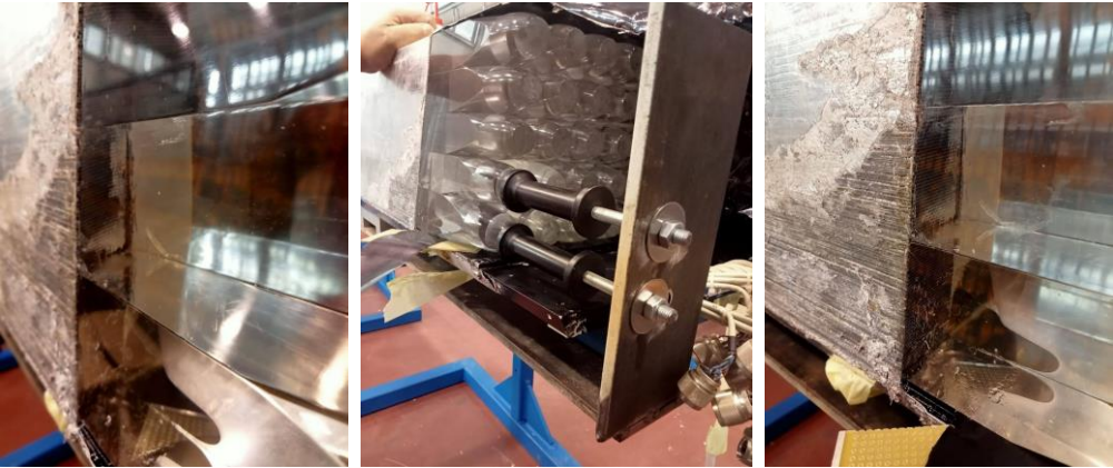
Gluing of light-guides and refurbishing of PMT support plate (1 module)
