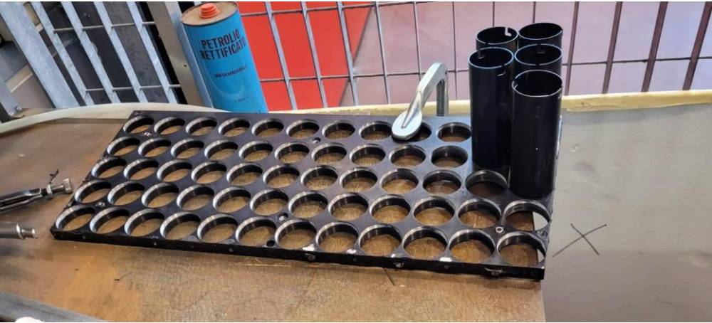
Gluing of light-guides and refurbishing of PMT support plate (1 module)
