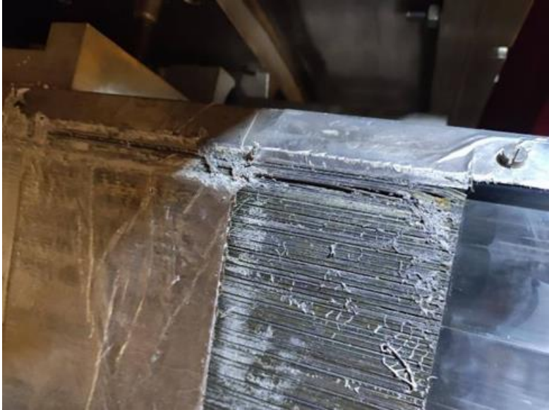
Gluing of delaminated modules (25%) after test of adhesives on Lead-fibres mock-up
