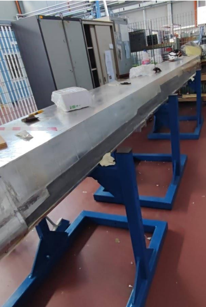
Gluing of light-guides and refurbishing of PMT support plate (1 module)
