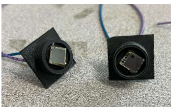
(Left) 3D-printed holder with soldered SiPM and electrical connections. (Right) Mounted SiPM holder in a lateral exit of the Horiba spectrometer/monochromator.
