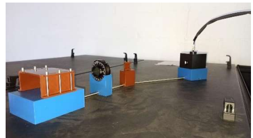
Figure #5: Shows the proposed setup for the reflectivity measurement. From left to right: laser support, polarizer, sample holder, and integrating sphere.
