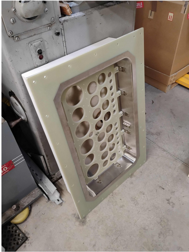
Test chamber with DAT support plate
