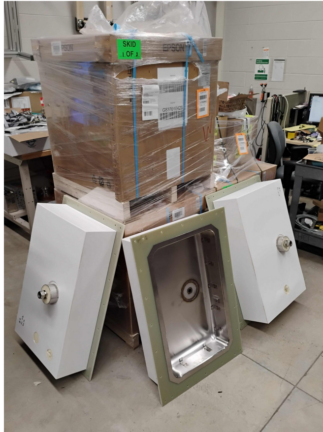
Six test chambers welded and insulated
